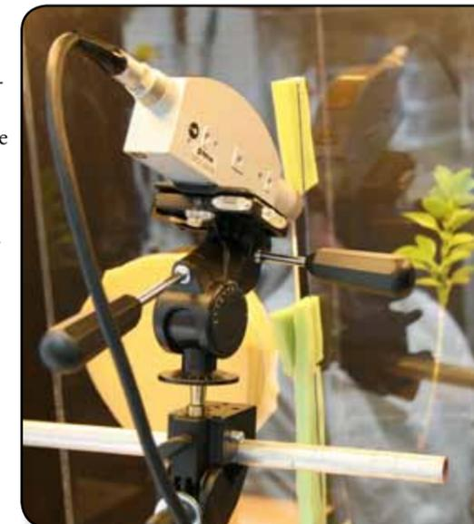
A Laser Doppler Vibrometer uses a laser beam aimed at a GWSS to record the super-low frequency sounds it makes, which are then recorded by a computer.
