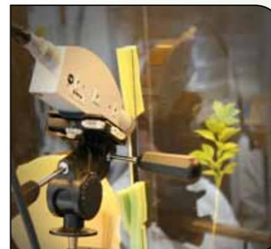
A laser-Doppler vibrometer is pointed at a single GWSS to pick up the sounds it is making.
